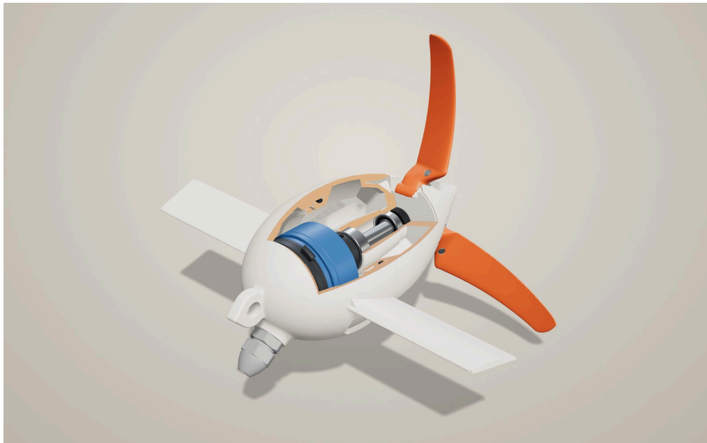
Figure 12: Cutaway render of the CAD assembly: generator replica (blue) on its carrier, claw coupling, shaft, 608 and 688 bearings, lip seal, and the v2 cable gland in the nose.
